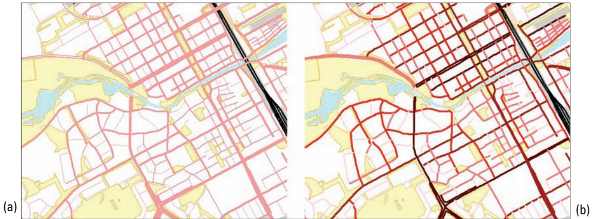
Figure 2. Visual variables for depicting multiple QL query results for linear features: a) size b) color value.
